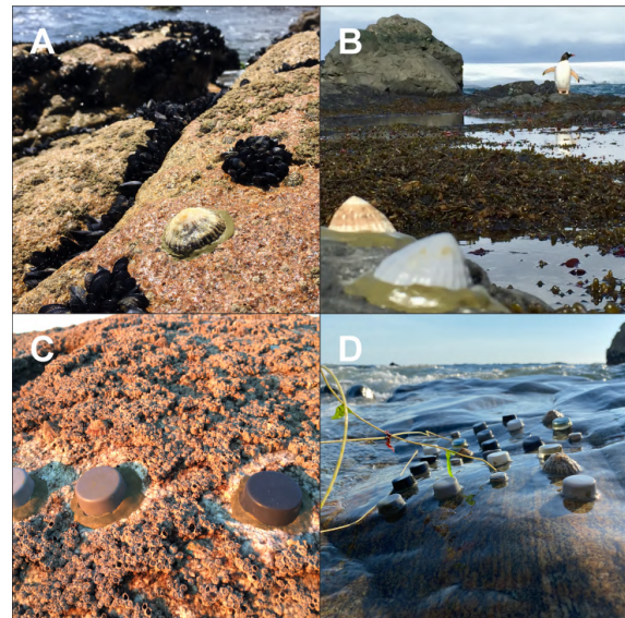
Figure 17. A – a robotlimpet with a real limpet shell glued to the rock. B – a robotlimpet with a resin shell and another with a real shell deployed in Antarctica. C – 27 mm EnvLoggers (as those in Fig. 2 B) but with different shades of gray. D – range of colors and shapes being tested on the field.
