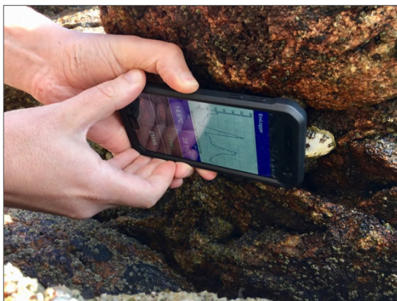
Figure 1. Temperature data being retrieved from an EnvLogger in the field. This particular EnvLogger was previously encapsulated in a limpet shell and permanently
