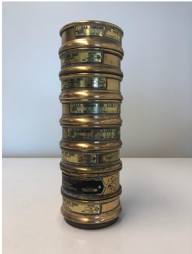
Figure 2. Example of sieve tower used to obtain size-fractionated epifaunal abundances.
