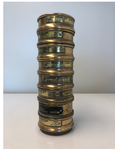
Figure 2: Example of sieve tower used to obtain size-fractionated epifaunal abundances.
