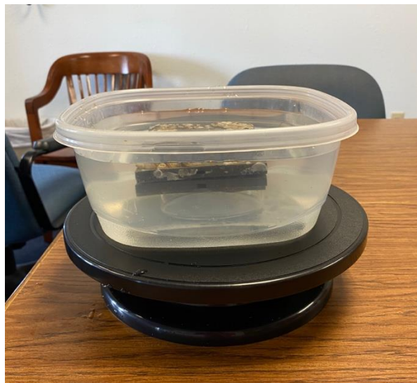
Figure 2. Submersed tile in photography container on turntable.
