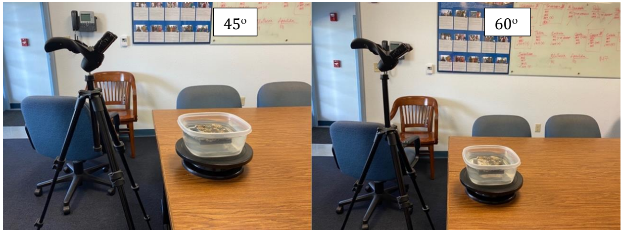
Figure 4. Tripod with camera aimed at panel on turntable.
