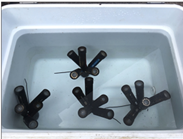
Figure 2.3. Photograph showing four clusters of five Onset U22 data loggers soaking in a warm bath used for a calibration check.
